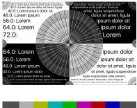
**Focus** provides easy reference for focusing and adjusting key stone.
